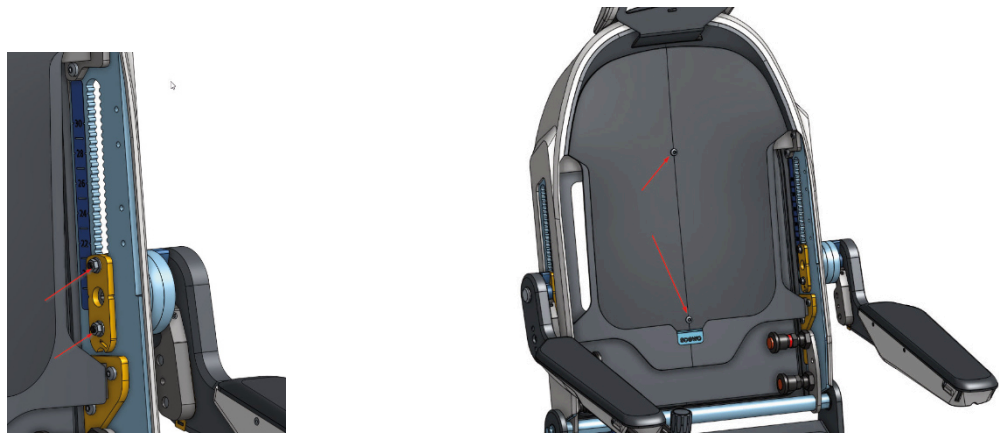
(a) Screws to be loosened in order to remove the arm support
