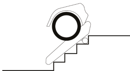
Figure 60. Premature detection of the end of stairs in the middle of the stairs
